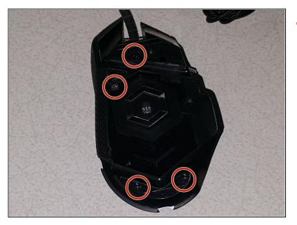
Remove the four Phillips screws holding the two halves of the mouse together.
