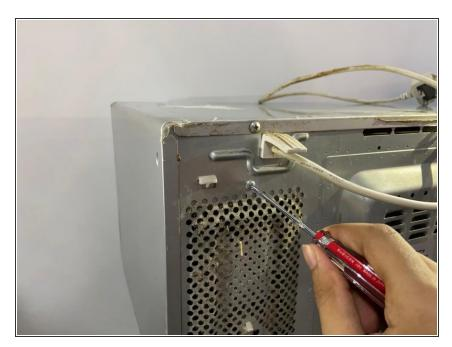
Remove the four 20 x 3" screws on the rear side of the microwave using a Phillips #0 screwdriver.
