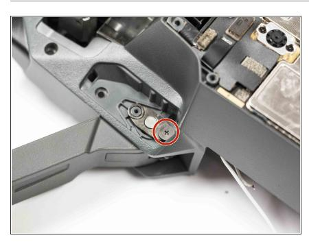
Remove the Phillips head screw below the arm to be replaced
