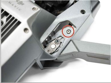
Remove the two 1.5mm hex screws under the cover
