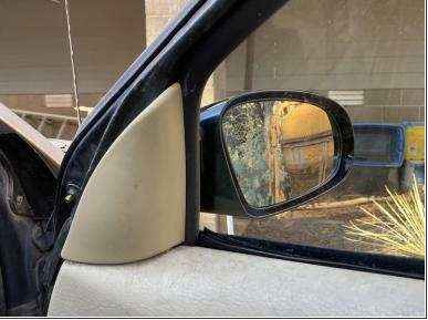
Replace the plastic panel by snapping it back on.
