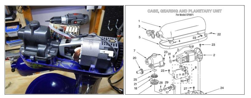
Install the new motor W10247536 number #2 and test it after you reinstall all the screws holding it down. Remember to hook back up the electrical wires before testing the KitchenAid Pro Series Stand Mixer Motor.
