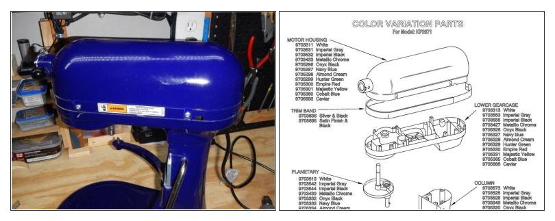
• There are four screws holding the motor in place remove them and lift the motor out. Remember to disconnect the wiring connector before you remove the mixer motor from the body.
