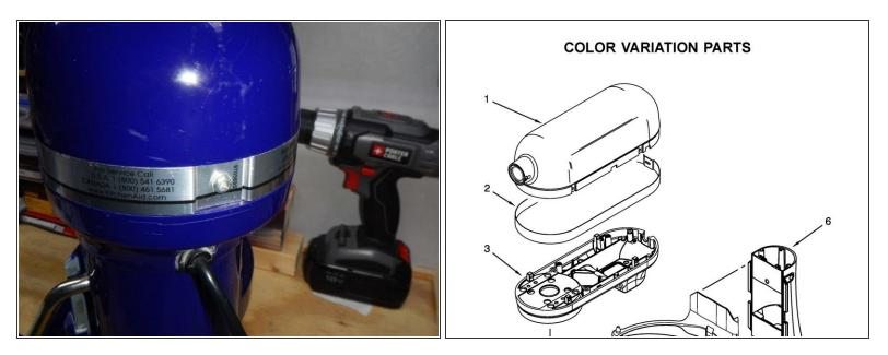
Remove the lid there is one screw at the back holding the band onto the mixer, and four screws holding the lid on.
