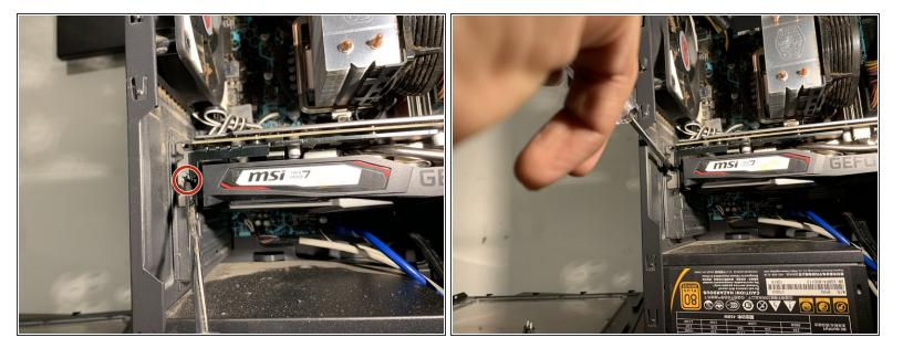
• Using a Phillips #1 screwdriver, remove the screw holding the graphics card to the case.
