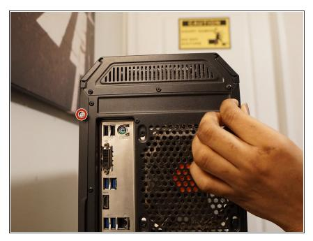
Remove the two screws holding the cover to the rest of the computer case.
