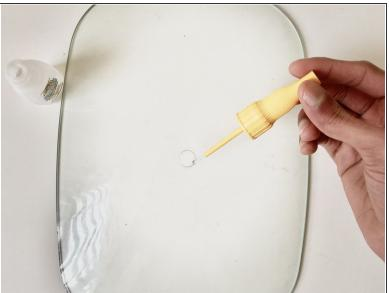
Apply super glue around the hole of the handle.
