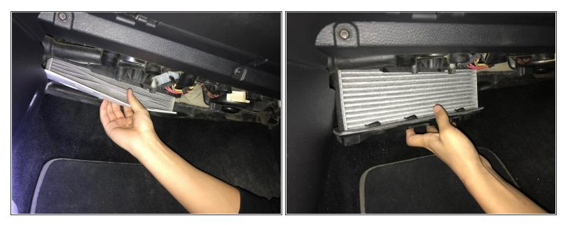
• Take out the filter carefully (it may contain dust) and replace it with a new filter.
