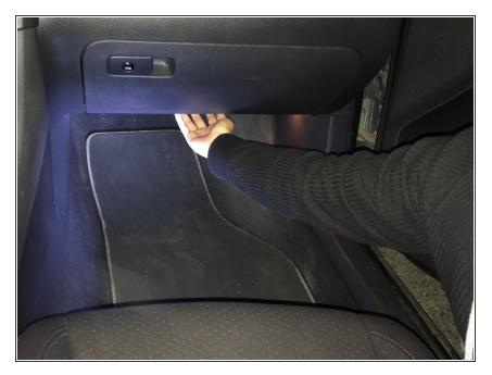
Locate the filter (it should be located in the lower part of the glove compartment)
