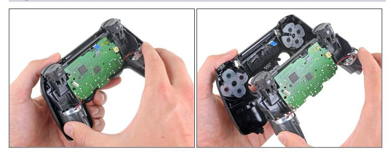
Separate the motherboard and midframe assembly from the front panel.
