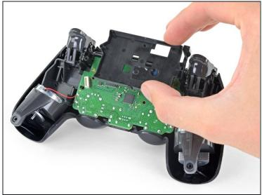
• Remove the battery bracket.
