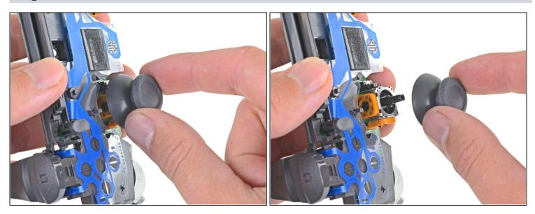
• Pull the left joystick cover straight off the joystick module to remove it.
