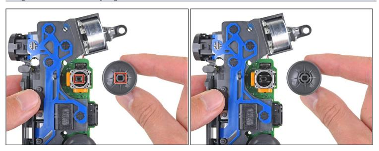
During reassembly, ensure the new joystick covers properly align with the shafts on the joystick modules before pressing them into place.
