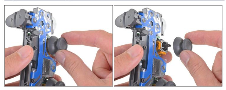
• Pull the right joystick cover straight off the joystick module to remove it.
