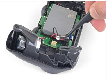
• Use a pair of tweezers to pull the battery's power connector straight up from the motherboard.
