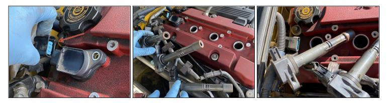
• Only unplug the last coil pack. Then pull all the coil packs out of the spark plug holes.
