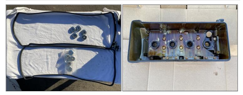
• Compare the old and new parts and make sure they are the same. Clean the inside of the valve cover with an old rag.
