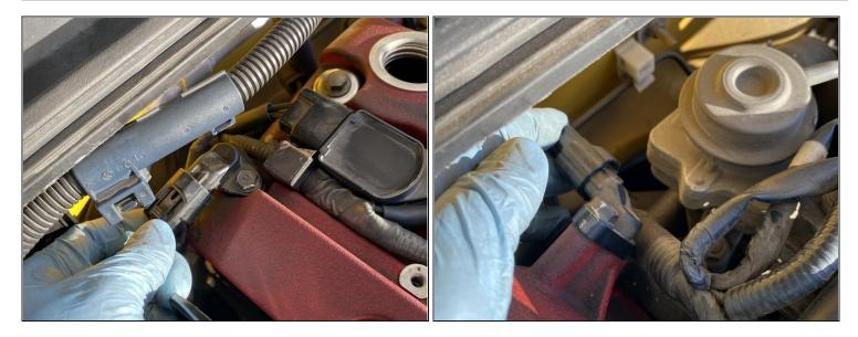
• Plug the two plugs back in on the back of the valve cover.
