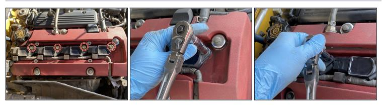
• Using a 10mm deep socket and a Torque wrench, remove the four 10mm bolts from all four coil packs.
