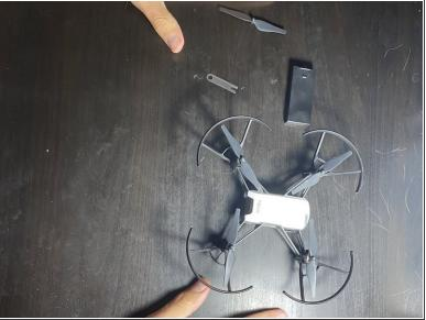
Next, remove the battery by grasping each side and pulling it out.
