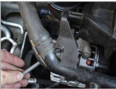
Using the 1/2 in. socket, remove the screws.
