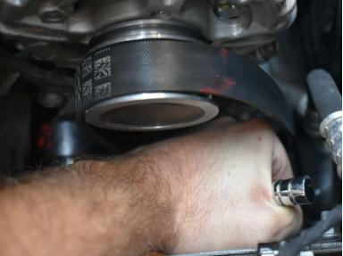
Using 11/16 in. socket, rotate clockwise to loosen the bolt
