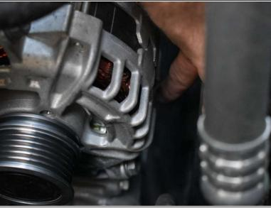
Locate the 4 screws holding the alternator in place two on the top and two on the bottom.
