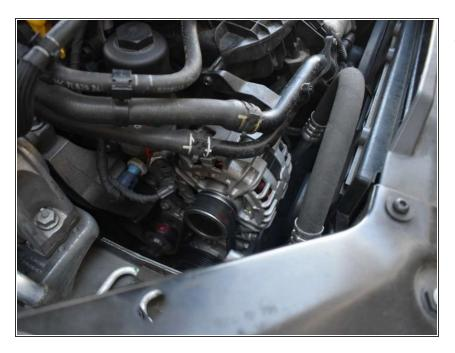
The alternator will be on the left side when facing engine
