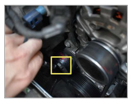
The belt loosening bolt is on the left, below the alternator.
