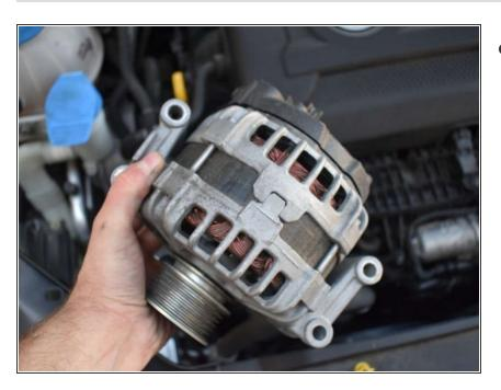
Take alternator out of engine by pulling to the left and out.
