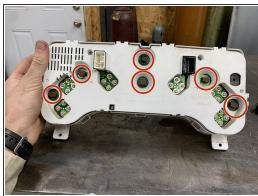
Remove the old light bulbs from the dash and replace them with the new ones. To do so simply twist the body of the light and it will pop right out. To install the new bulbs do the opposite. Push the body of the bulb flush with the mounting surface on the dash and then twist to hold it tight.
