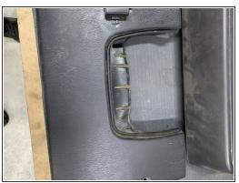
Remove the two screws that hold the second part of the dash cluster, then remove the dash cluster.
