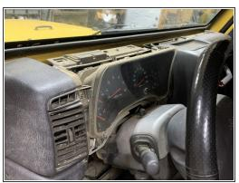
Now that all four screws holding the dash on are visible, remove them to allow the dash to come
