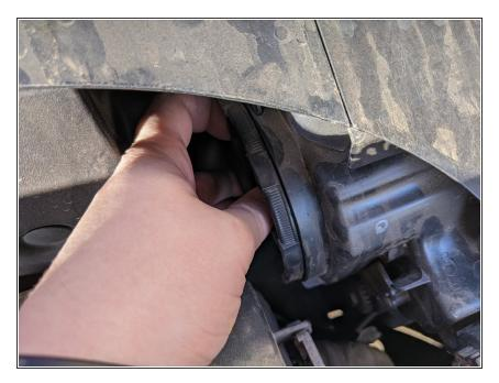
Remove the bulb cover cap by rotating it counter-clockwise until it is fully detached.
