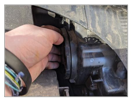
Locate the bulb cover cap which can be found under the hood and directly behind the headlight.
