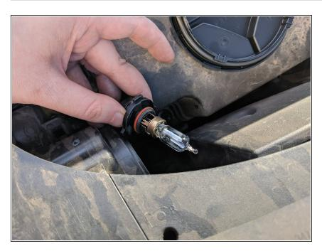
Remove the old bulb by rotating counter-clockwise until it is detached, being careful not to drop the bulb into the hood of the vehicle.
