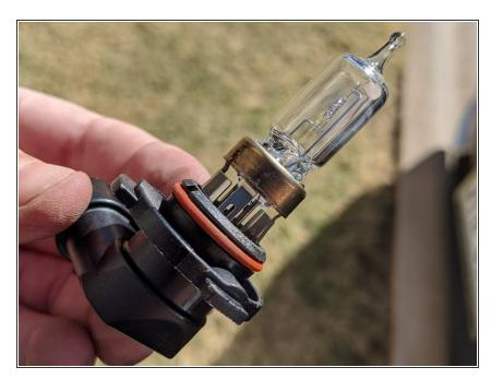
Prepare your replacement XtraVision Fog Light/Headlight Bulb 9005XV-2 for installation by removing it from the packaging and ensuring that the bulb is not broken.
