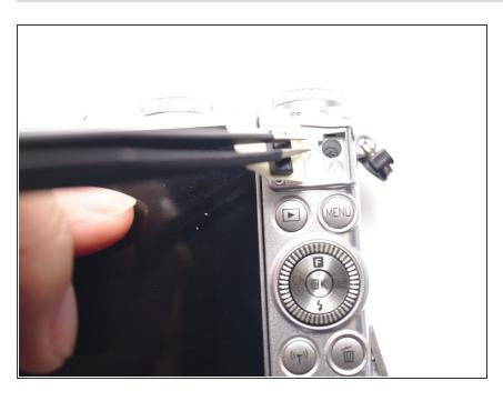
Peel here and remove 1 screw within.
