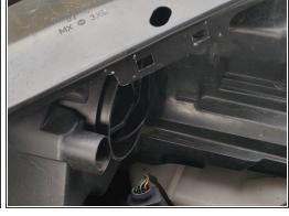
Locate the plastic dust cover behind the burnt headlight and gently remove it. If the cover is stuck, you can use a screwdriver to pop it out.
