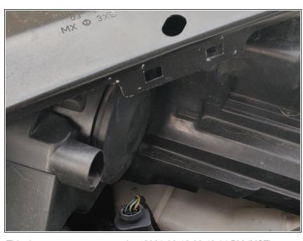
Reapply the dust cover and close the hood of the vehicle.
