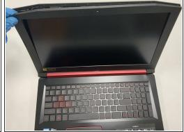
Pry open the plastic bezel around the screen by going around all four sides with a plastic opening tool.
