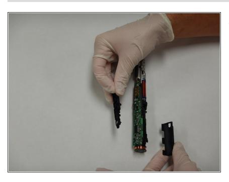
Remove the rubber covers from the circuit board and battery.
