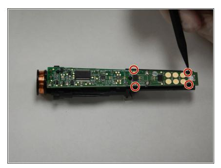
Carefully free the top end of the circuit board from the plastic clips holding it in place.
