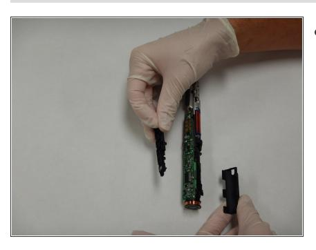
Remove the rubbers covers from the circuit board and battery.
