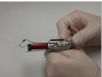
Gently bend and position the brackets to remove the motor.
