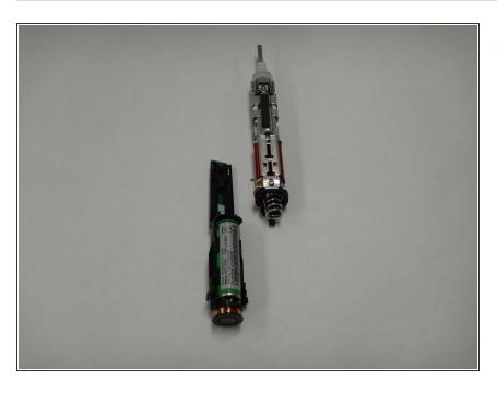
Slide and separate the two components of the internals from each other.
