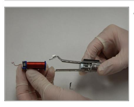
Remove the motor and replace.
