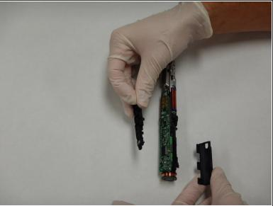
• Remove the rubber covers from the circuit board and battery.
