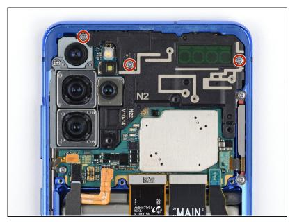
Use a Phillips #00 screwdriver to remove the three 4 mm-long screws securing the upper midframe.
