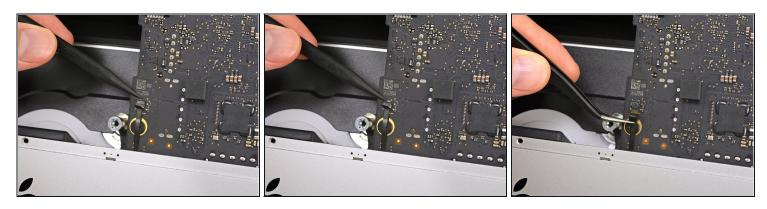
• Use the tip of a spudger to flip open the retaining flap on the microphone ribbon cable <u>ZIF socket</u>.
