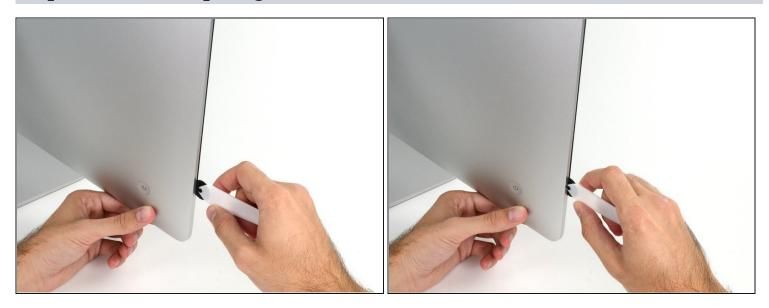
• Starting on the left side of the display, near the power button, insert the iMac Opening Tool into the gap between the glass panel and the rear enclosure.
