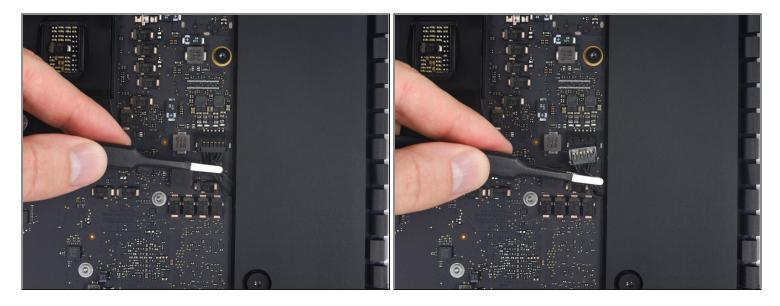
• Use a pair of tweezers or your fingers to pull the right speaker cable connector straight down and out of its socket on the logic board.
