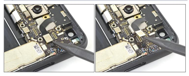
• Disconnect the earpiece speaker connector from the motherboard.
