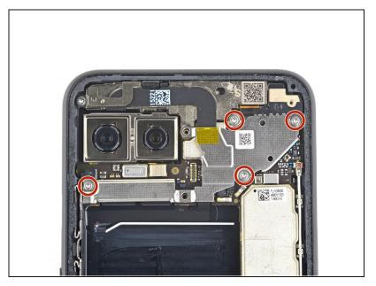
Use a T3 Torx driver to remove the four 4 mm screws securing the camera connector cover.
