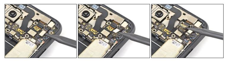
• Using the pointed end of a spudger, pry the camera and sensor connectors straight up from the motherboard.
