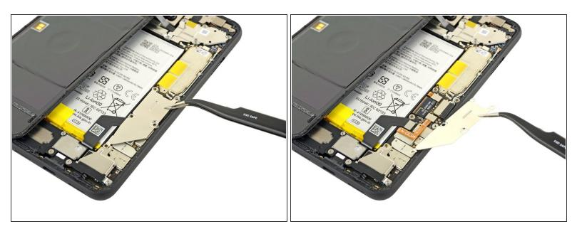
Use a pair of tweezers to remove the battery connector shield.
