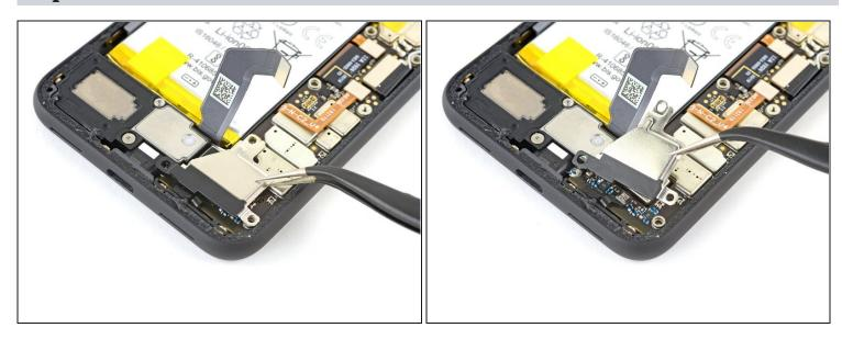
• Use a pair of <u>tweezers</u> to remove the vibration motor shield.
