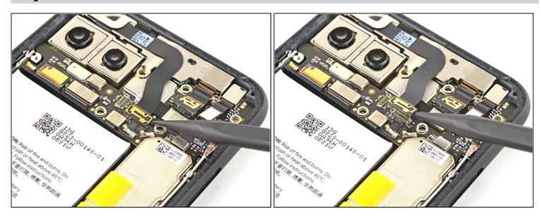
• Disconnect the laser module connector.
