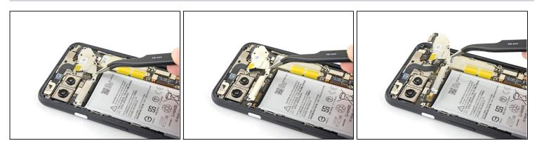
• Using a pair of <u>tweezers</u>, tilt the camera cover up and slide it out of the retaining slot on the upper right corner of the phone to remove.
