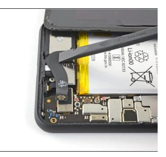
• Using the flat end of a spudger, gently fold the battery cable over so it doesn't accidentally make contact during the rest of your repairs.
