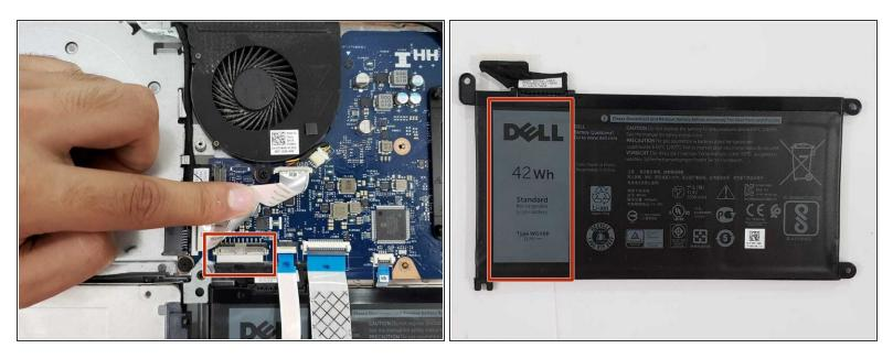
• Disconnect the battery connecting cable from the laptop by sliding it out.
