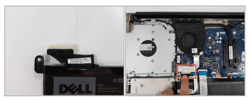
• Attach the cable for the new battery to the laptop by sliding the cable into the port.
