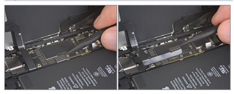
• Use the point of a spudger or a fingernail to disconnect the front panel sensor assembly connector.
