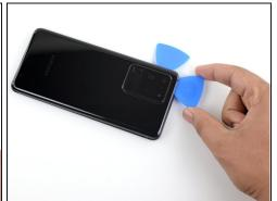
⚠ The glass near the corners of the back cover is curved and very susceptible to cracking. Be gentle during this step to prevent damaging your back cover.
