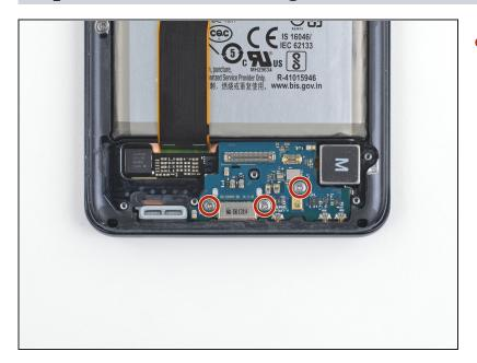
Use a Phillips #00 screwdriver to remove the three 3.7 mmlong screws securing the USB-C port and daughterboard.
