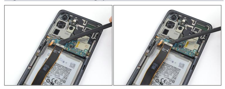
• Pry up and disconnect the main display flex cable from the motherboard.
