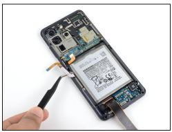
Gently peel up and bend the display and left 5G antenna flex cables out of the way of the motherboard and battery.
