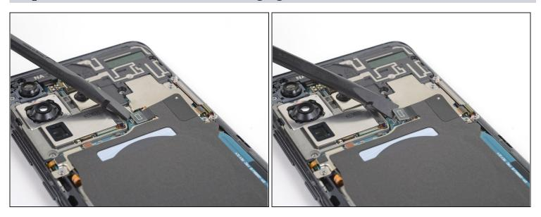
Use a spudger to pry up and disconnect the wireless charging coil connector.
