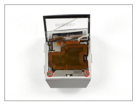
Remove the two Torx T2 screws
