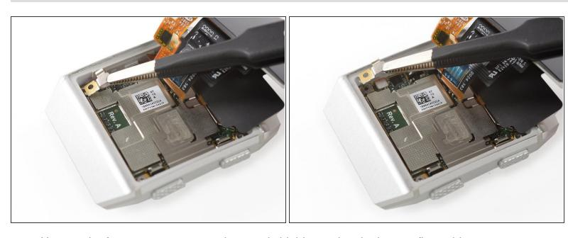
Use a pair of tweezers to remove the metal shield covering the battery flex cable.
