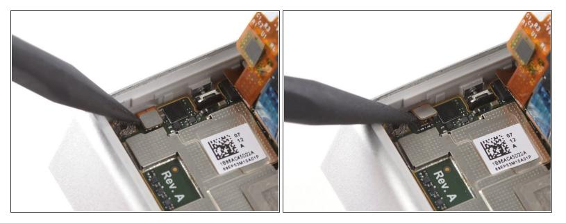
Use a spudger to pry up and disconnect the battery flex cable.
