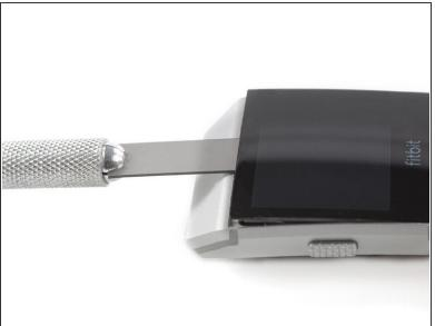
Use a technician's razor with a flat blade to pry up the top edge of the display and create a small gap.
