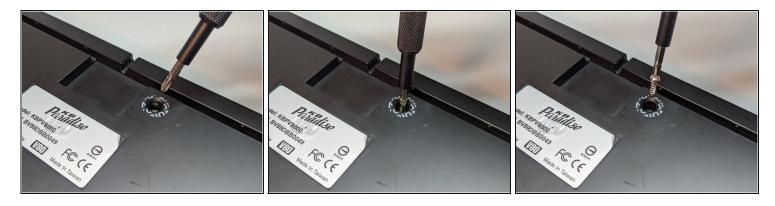
• Use a Phillips #1 Screwdriver to remove the 10 mm screw.
