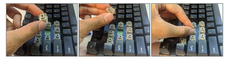
• Insert a new key switch into the well with pins corresponding to that of the PCBs.
