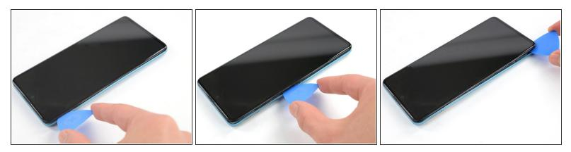
Slide the opening pick from the top left corner to the bottom left corner to release the left side's plastic clips.
