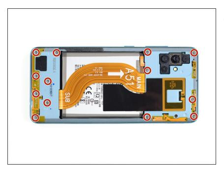
Remove the thirteen 3 mm Phillips #00 screws securing the midframe.
