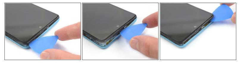
Slide the opening pick along the top edge to release the top plastic clips.
