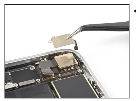
• Remove the rear-facing camera bracket.
