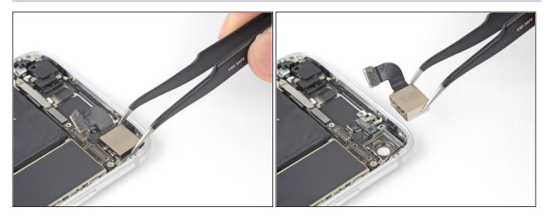
• Remove the rear camera by lifting it straight up out of its recess.
