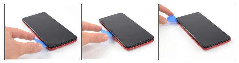
Slide the opening pick from the top left corner to the bottom right corner to release the remaining clips.
