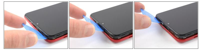
Slide the opening pick from the top left corner to the top right corner to release the plastic clips.
