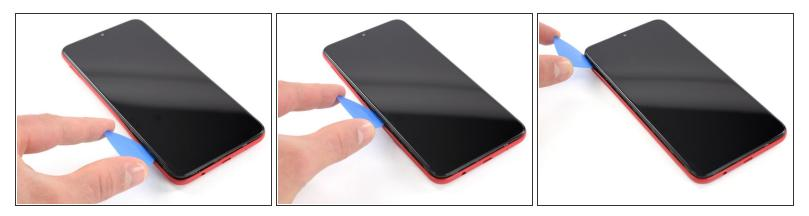
Slide the opening pick along the left edge to the top left corner of the phone, to release the clips.
