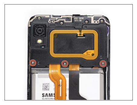
Remove the three Phillips #00 screws (3 mm length).
