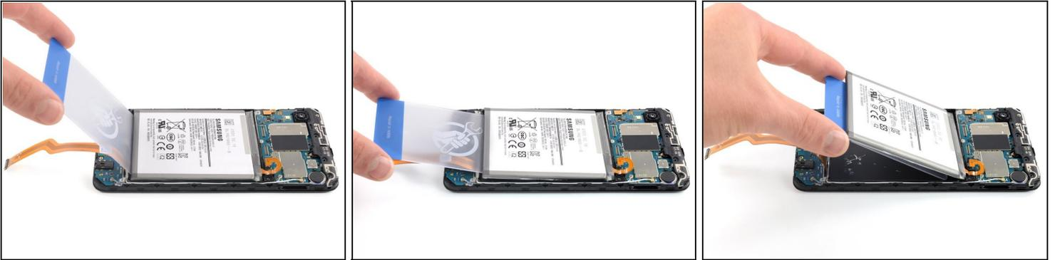
**⚠ Try your best not to deform the battery during this process. Soft-shell lithium-ion batteries can leak dangerous chemicals, catch fire, or even explode if damaged. Do not use excessive force or pry at the battery with metal tools.**
