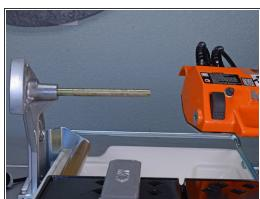
Pull the entire cutting head straight off the shaft holding it in place.
