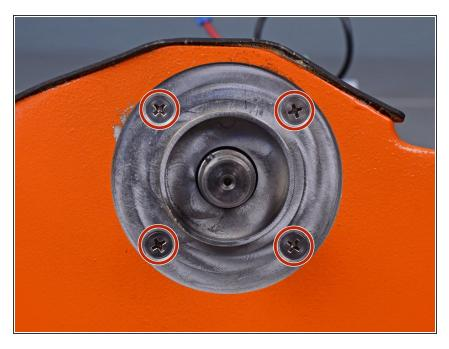
Remove the four Phillips #2 screws holding the motor in place.
