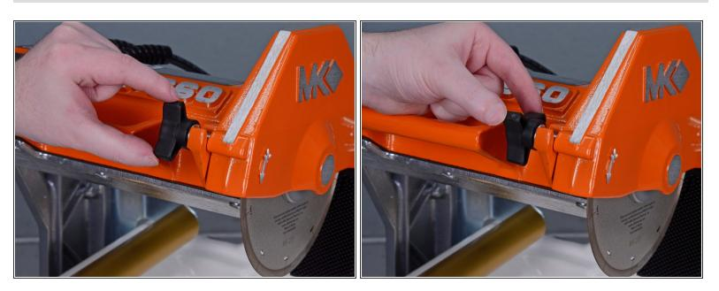
Loosen the plastic knob holding the blade cover in place.
