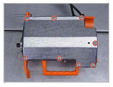
Remove the eight Phillips #2 screws on the underside of the cutting head.
