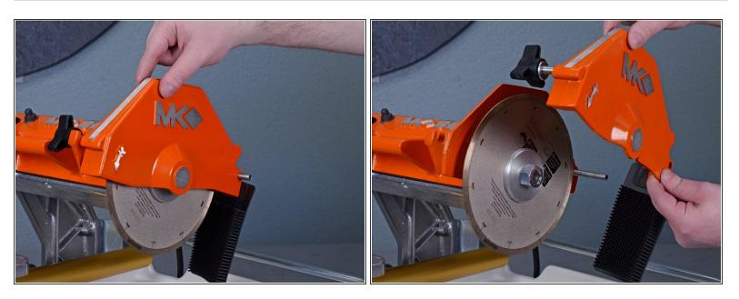
Pivot the blade cover up and pull it off the shaft.
