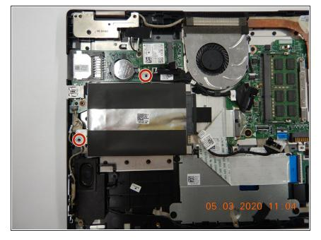
Using the Phillips #000 screwdriver, remove two 3mm screws from the hard drive frame.
