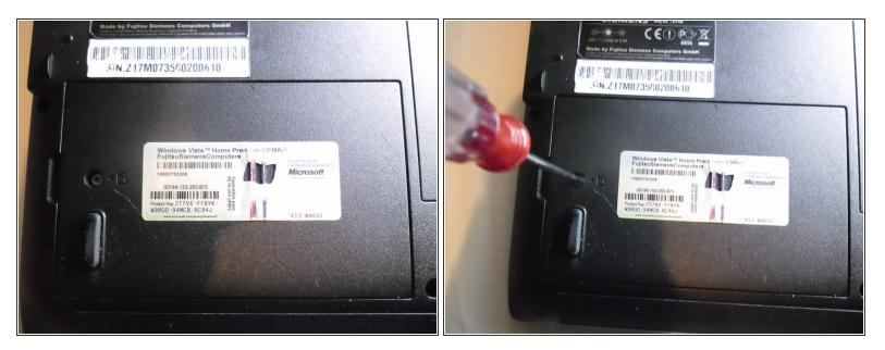
• Locate the hard drive cover and remove the screw.
