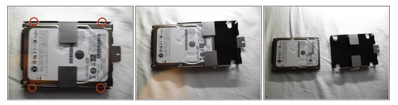
• There is a screw on each corner of the hard drive bracket. To take the hard drive out of its bracket you need to remove the 4 screws.
