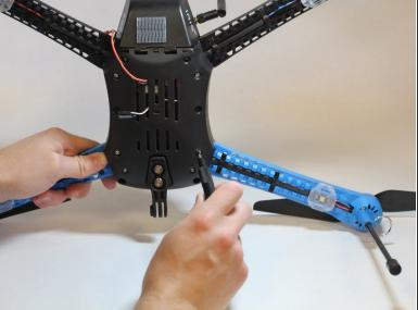
Remove the eight 11mm screws attaching the underbody of the drone using the 2mm Hex screwdriver/key.
