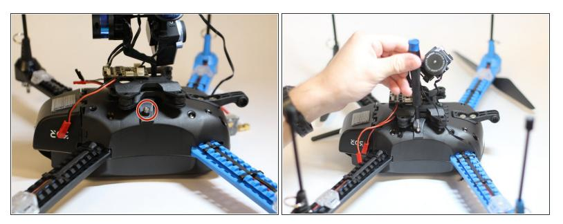
Unscrew the 16 mm screw attaching the gimbal mount to the body of the drone using the 3 mm Hex screwdriver/key.
