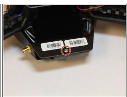
With the back plate off, remove the three 4mm screws using the Hex 2 mm screwdriver. These secure the top plate to the drone assembly.
