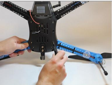
Remove the eight 11mm screws attaching the underbody of the drone using the 2mm Hex screwdriver/key.
