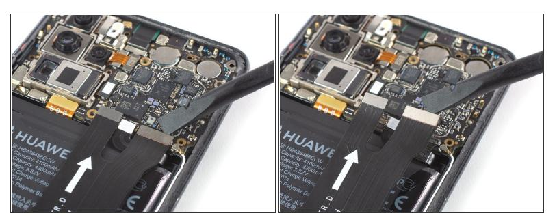
• Use a spudger to pry up and disconnect the right main flex cable connector from the motherboard.
