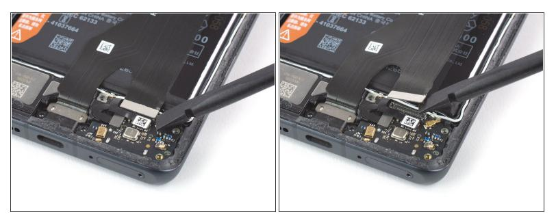
• Use a spudger to pry up and disconnect the main flex cable connector from the daughterboard.
