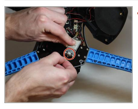
Lightly pull the wire to disconnect it from the RX Transmitter.
