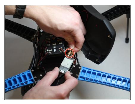
Using your fingers, gently twist and disconnect the gold part on the cable attached to the RX Transmitter.
