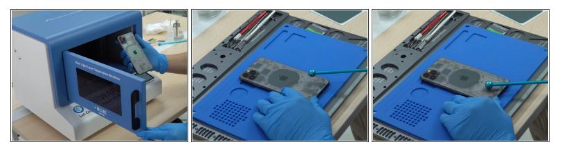
• Once the laser is finished, take out the phone and give the back glass a little tap with a focal length rob. The back glass would appear with some cracks, it would be easier to separate.
