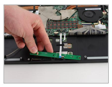
Remove the trackpad circuit board by holding one end and gently lifting it upwards.
