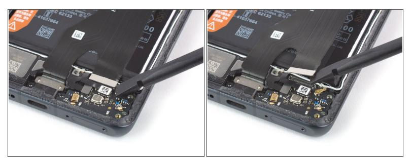
Use a spudger to pry up and disconnect the main flex cable connector from the daughterboard.
