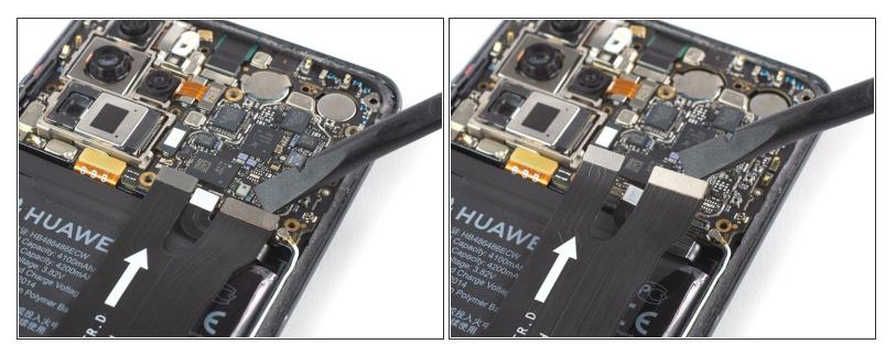
Use a spudger to pry up and disconnect the right main flex cable connector from the motherboard.
