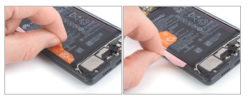
Peel the orange adhesive strip labeled with a 2 off the battery. The orange adhesive tape will rip along a small perforated line.
