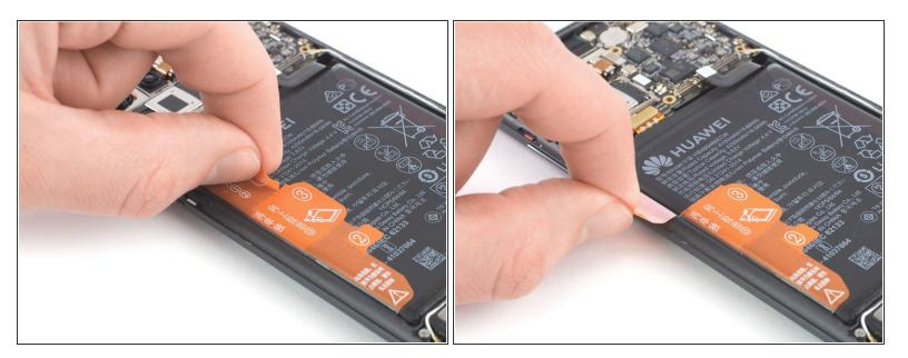
Peel the orange adhesive strip labeled with a 1 off the battery. The orange adhesive tape will rip along a small perforated line.
