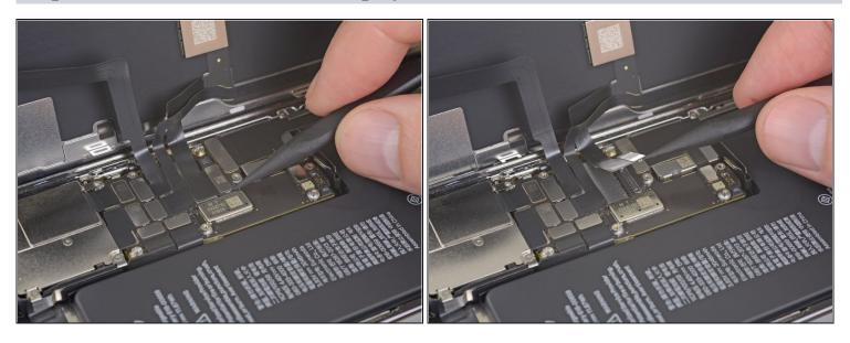
• Use a spudger or a fingernail to disconnect the OLED panel cable connector.
