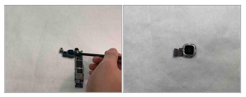
Once the motherboard is removed, use the spudger to disconnect the rear camera from the motherboard.
