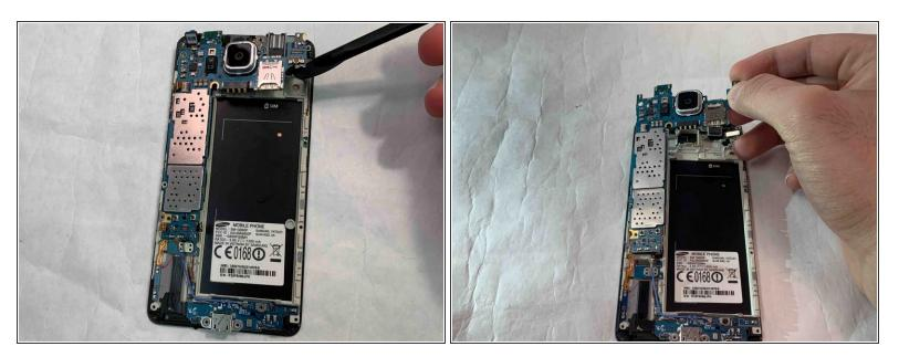
• Using your hands or a spudger, lift up and remove the motherboard.
