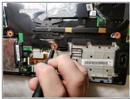
• Remove the ten 5mm screws holding down the motherboard using the Phillips #0 screwdriver.
