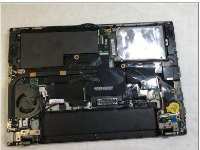
Remove the two rubber stoppers from where the battery previously was.
